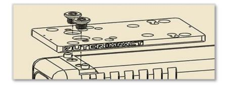
Note: The adapter has an intentional curve. This curve will flatten out when mounted. Utilize blue liquid thread locker upon final installation of all threaded fasteners.
